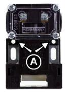
After mounting and adjusting the operating claw you can fix the switch by 2 drill holes (A) with pins ( $\emptyset$  4mm) against rotation.
