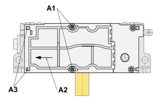
Unscrew cover screws (A1) min. 4 mm up to max. 7 mm. Then move the cover (A2) in the direction of the cable entry to release the cover from the retaining hooks (A3). The cover can now be removed.
