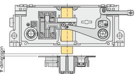
Y-dimension = dimension between completely drawn in latch bolt and upper edge latch plate nominal dimension Y=3.5 mm and nominal dimension  $X \ge 5$  mm
